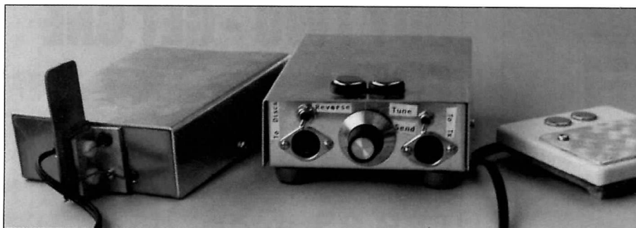
Selection of touch keyers. Left: Vertical blade iambic keyer. Centre: iambic keyer with built-in electronics. Right: Touch pads. The operator rests the wrist on the rectangular pad and keys by touching the buttons.
